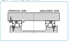
Figure A-14 No Reference Surface on Adjustable Side
